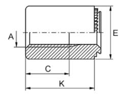
Female thread A = M4Height K = 25Min distance to edge = 4.0Outer diameter E = 8Plate thickness = 1.5 to 2.3Recommended bore diameter +0.05 = 5.00Thread length = 8.0
